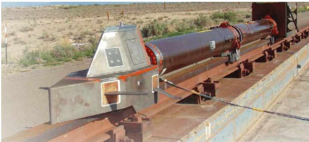
A monorail dry-run test at Holloman AFB in July 2013 had no payload and used three representative carbon-epoxy panels mounted on the top and sides of the sled
